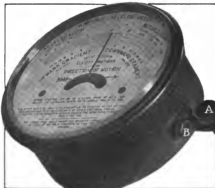
Partial side view of instrument, showing needle lock B and leveling screw A
